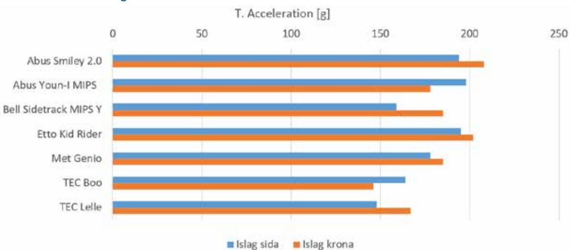
Figure 1. Shock Absorption measuring linear acceleration
